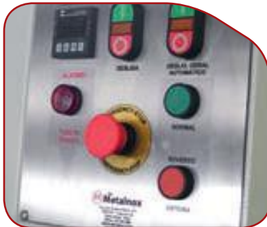
Reverse driving of the fabric and transfer, allowing for correcting their path in case they are fed-in misaligned
