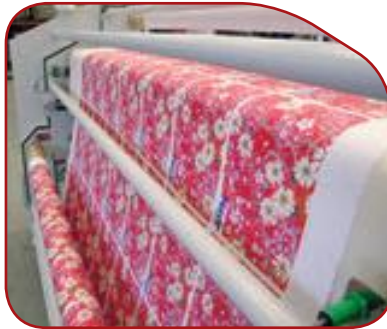
Even temperature and fabric-tensioning system capable of feeding the fabric duly centered.
